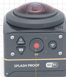
**CONTROLS** All the Pixpro SP360's controls are grouped on one side of the cube, making it nice and easy to see what's going on. The on/off button doubles up to switch between Modes, then a menu button to access settings. The big Rec button is easy to find in the middle and also confirms settings, with the Wi-Fi button to its right.
